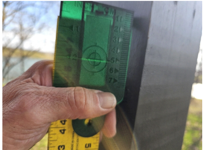
46 5/8 lake side. This point is 1 1/8" lower than center reference. This should be monitored to make sure footings are not moving.
